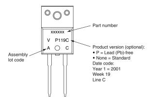
Example: This is a xxxxxx with assembly lot code AC assembled on WW 19, 2001 in the assembly line "C"
